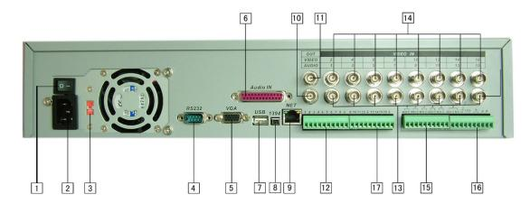
1, power switch 2, power plug 3, 220V/110V shift switch 4, RS232 connection
